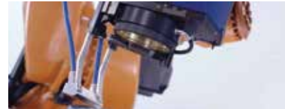
Remote laser welding 3D
