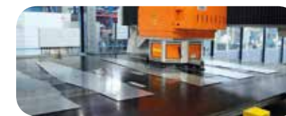
Laser welded blanks
