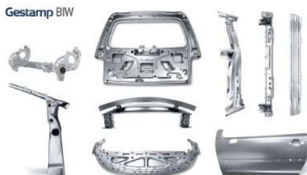
Chassis comprises systems, frames and related parts, such as front and rear axles and links, control arms and integrated links, which are used to create the essential lower body structure and carry the load of the vehicle. These structures are essential for the vehicle's performance and safety, in particular affecting vehicle noise levels, vibrations, handling and behavior in the event of an impact.
